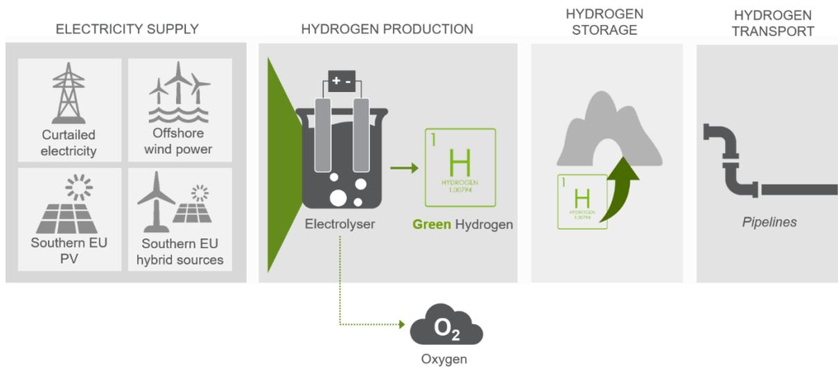
**Figure 5. Production pathway for green hydrogen produced through electrolysis**
