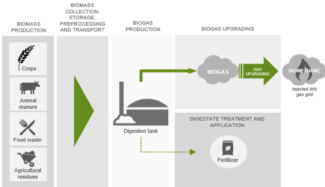
**Figure 3. Production pathway for biomethane produced through anaerobic digestion**
