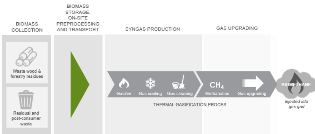
**Figure 4. Production pathway for biomethane produced through thermal gasification**
